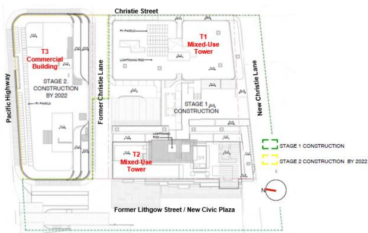
Figure 27. Construction stages (Source: PTW).
