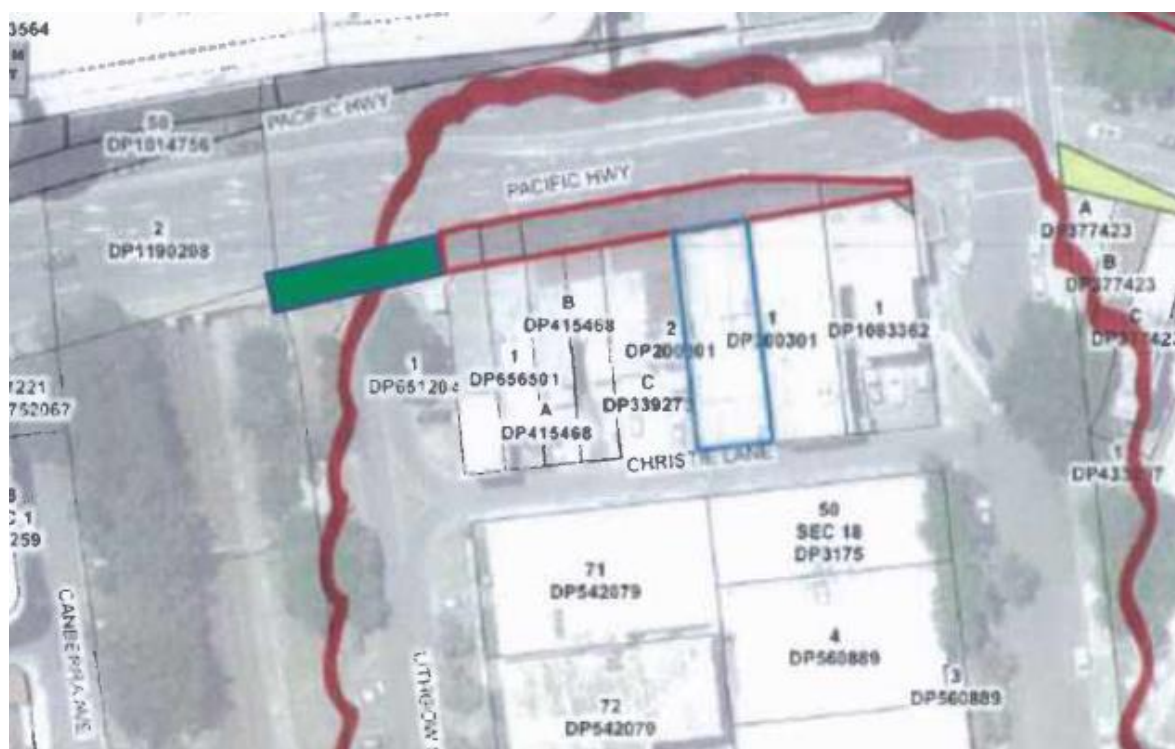
Figure 76. RMS land dedicated as 'road' along the Pacific Highway frontage.
