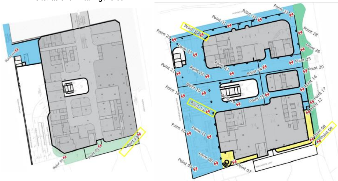
Figure 69. Study point locations at Lower Ground Floor (left) and Ground Level (right), and showing the four (4) locations, which exceed the safety criterion (Source: Report by Windtech).
